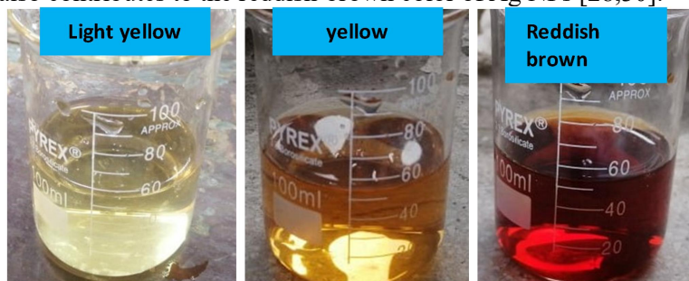
Figure 1: Color of nanoparticle solution after (a) 5 min (light yellow), (b) 10 min (yellow), and (c) 15 min (reddish brown)
