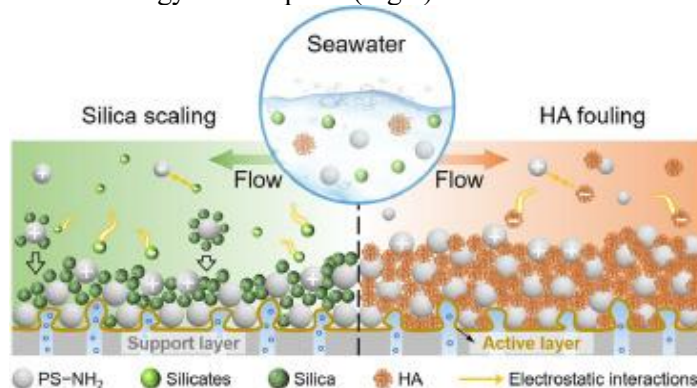
Figure 3: Impact of nanoplastics on membrane scaling and fouling in the reverse osmosis desalination process [22]
