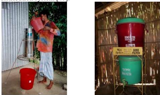
Figure 4 An Alcan filter in Azimpur village Bangladesh (left) and Sono arsenic removal filter (right)
