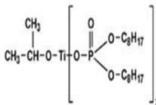
**Fig-2:** Isopropyl, tri (dicetyl) phosphonate titanate (Titanium 4, 2-propanolato, tris phosphonate-O)
