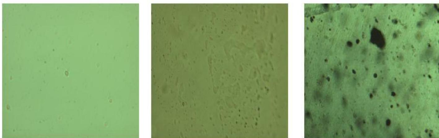
**Fig-6:** a) Polystyrene b) P.S with S.T c) P.S with S.T and Mg (OH)<sub>2</sub> (Magnification 630x)
