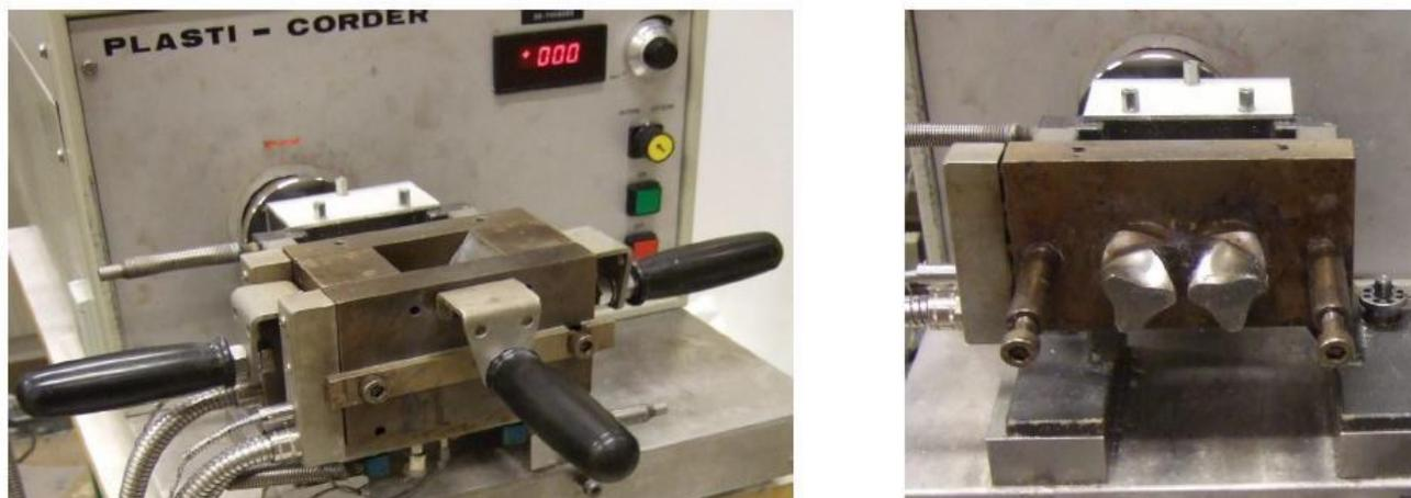
**Fig-3:** Brabender Plasticorder; (a) Mixer with control panel (b) Mixing screws
