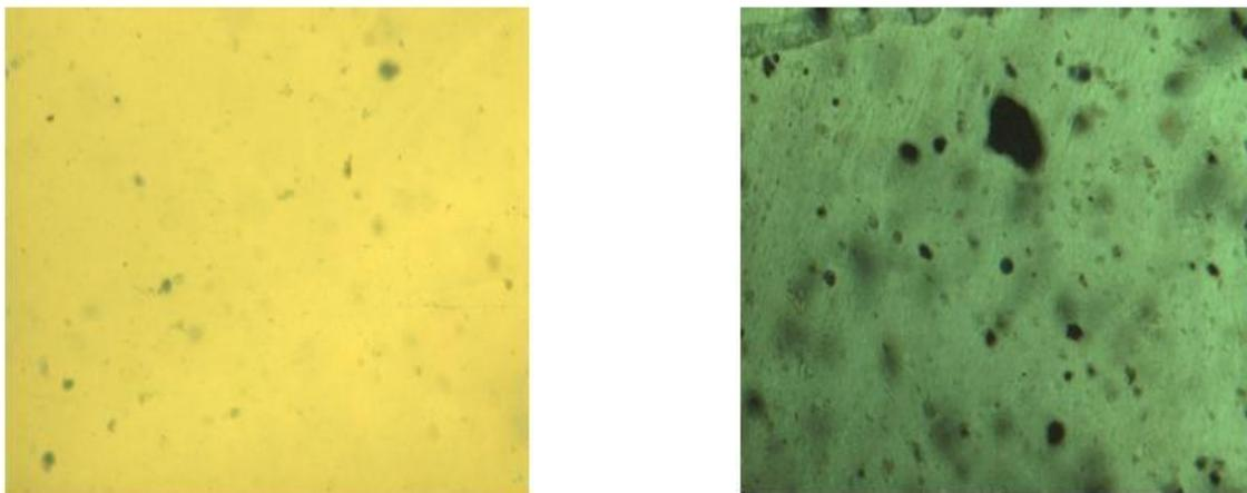
**Fig-8:** a) P.S, S.T, Alumina fibers, Mg (OH) 2 b) P.S, S.T and Al<sub>2</sub>O<sub>3</sub> fibers. (Magnification 630x)
