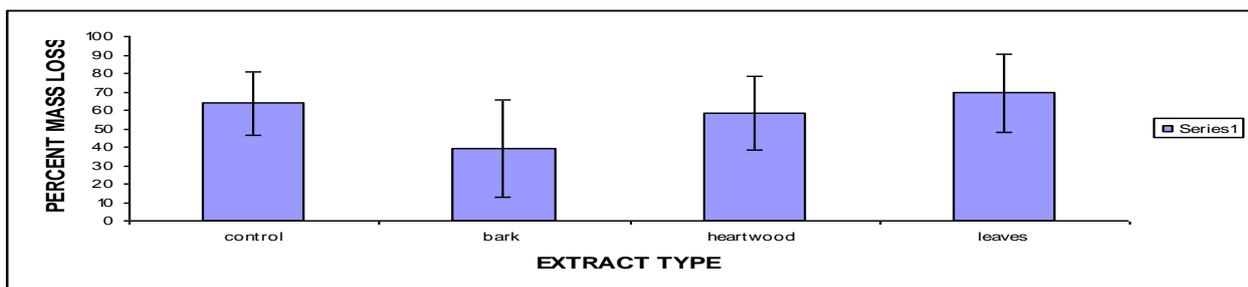
**Fig-4:** Percent mass loss of Bediwonua treated with Potrodom branch bark, heartwood and leaf water extractives at 0.5 g/ml after field exposure for 6 months. N=7, P=0.08,  $\alpha=5\%$ , F= 2.58
