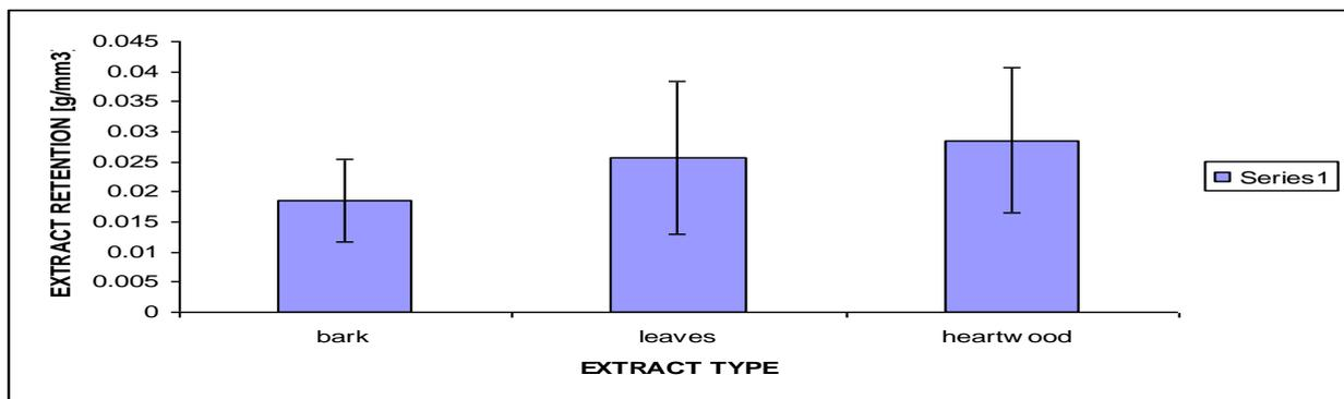
**Fig-2:** Retention of Potrodom branch bark, heartwood and leaf water extractives at 0.5 g/ml in Bediwonua after impregnation. N=7, P=3.12E-5,  $\alpha=5\%$ , F= 12.94.
