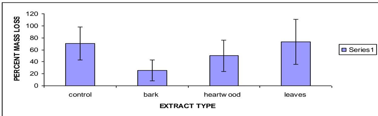
**Fig-3:** Percent mass loss of Chenchen treated with Potrodom branch bark, heartwood and leaf water extractives at 0.5 g/ml after field exposure for 6 months. N=7, P=0.01,  $\alpha=5\%$ , F=4.41.
