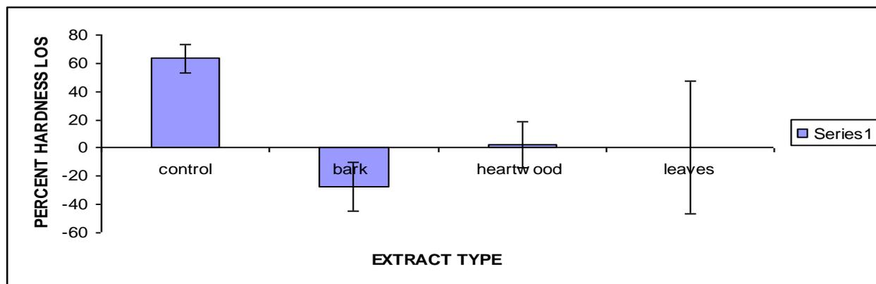
**Fig-5:** Percent hardness loss of Chenchen treated with Potrodom branch bark, heartwood and leaf water extractives at 0.5 g/ml after field exposure for 6 months. N=7, P=1.58E-5,  $\alpha$ =5%, F=14.20
