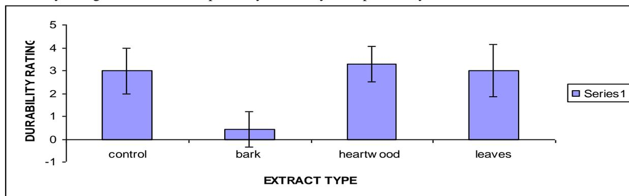
**Fig-7:** Visual durability ratings of Chenchen treated with Potrodom branch bark, heartwood and leaf water extractives at 0.5 g/ml after field exposure for 6 months. N=7, P=1.52E-5,  $\alpha$ =5%, F=14.27
