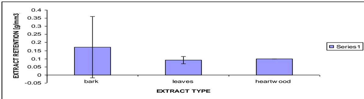
**Fig-1:** Retention of Potrodom branch bark, heartwood and leaf water extractives at 0.5 g/ml in Chechen after impregnation. N=7, P=0.02,  $\alpha=5\%$ , F= 3.82.
