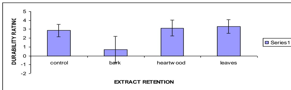
**Fig-8:** Visual durability ratings of Bediwonua treated with Potrodom branch bark, heartwood and leaf water extractives at 0.5 g/ml after field exposure for 6 months. N=7, P=1.95E-4,  $\alpha$ =5%, F=9.91
