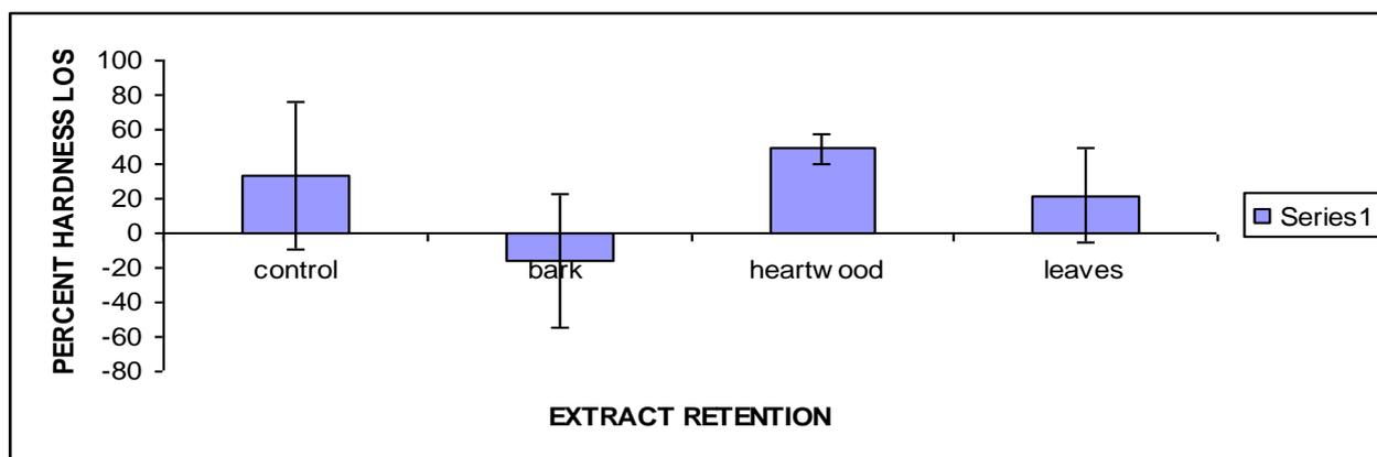
**Fig-6:** Percent hardness loss of Bediwonua treated with Potrodom branch bark, heartwood and leaf water extractives at 0.5 g/ml after field exposure for 6 months. N=7, P=0.01,  $\alpha$ =5%, F=5.06
