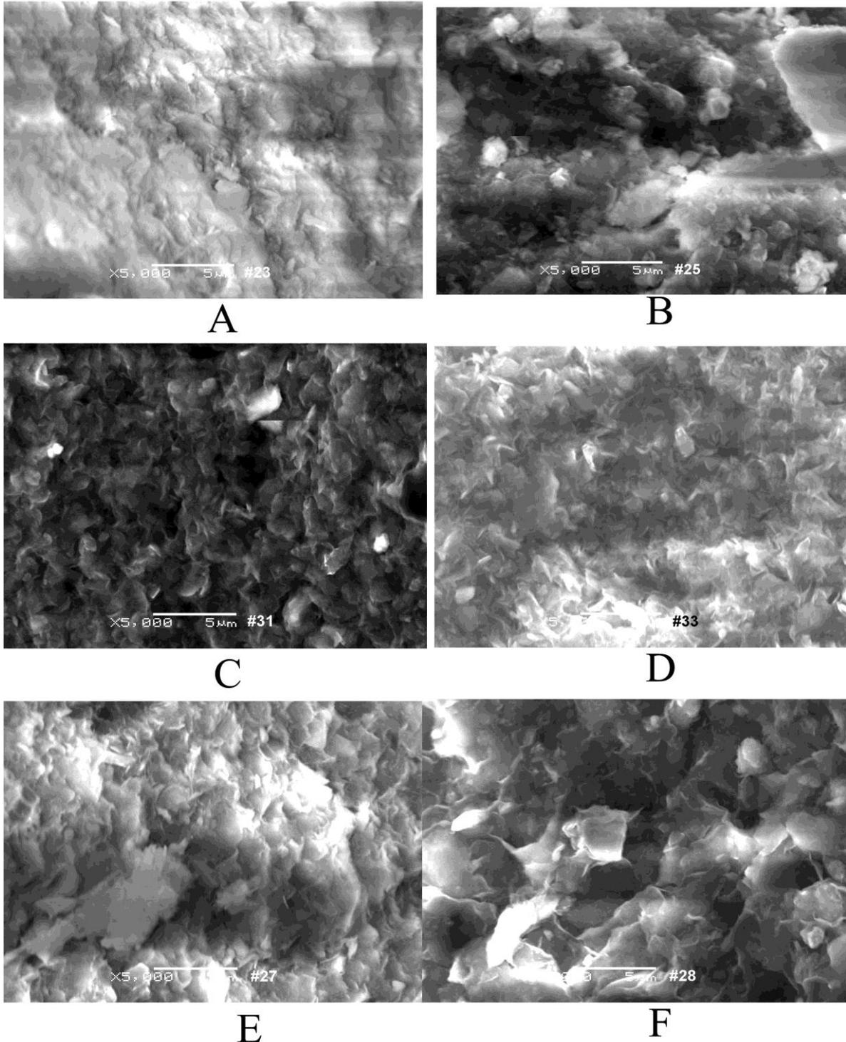
**Fig-3:** Scanning Electron Microscope images for clay samples of studied soils
