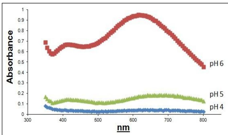
**Fig-3:** Spectra of Fe (II) complexed with Levodopa, pH 4.0, 5.0 and 6.0 buffer solutions. Fe (II) = 0.005 mmol, 10 fold ligand solution
