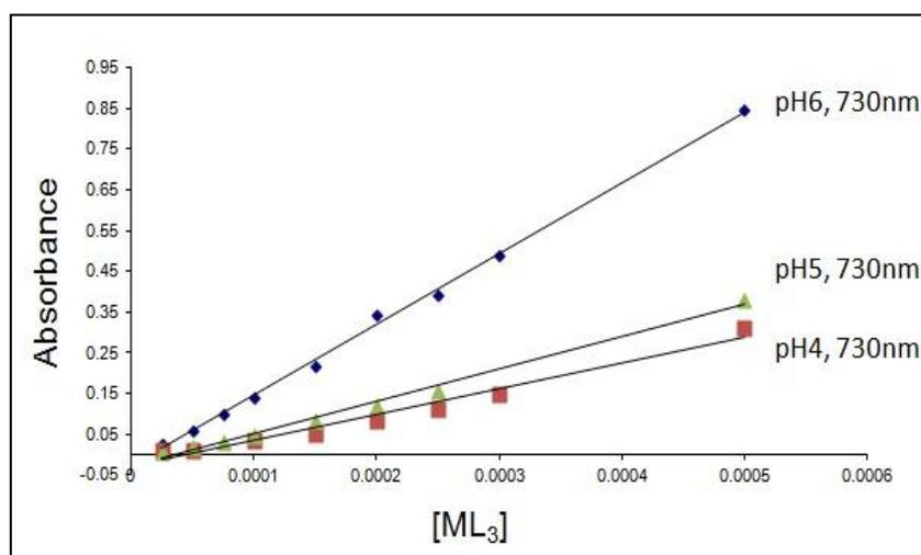
**Fig-5:** Molar Absorptivity of Fe (II)-Levodopa Complex, pH 4.0, 5.0 & 6.0,  $\lambda = 730nm$ .
