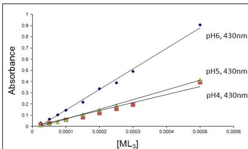
**Fig-4:** Molar Absorptivity of Fe (II)-Levodopa Complex, pH 4.0, 5.0 & 6.0,  $\lambda = 430nm$ .
