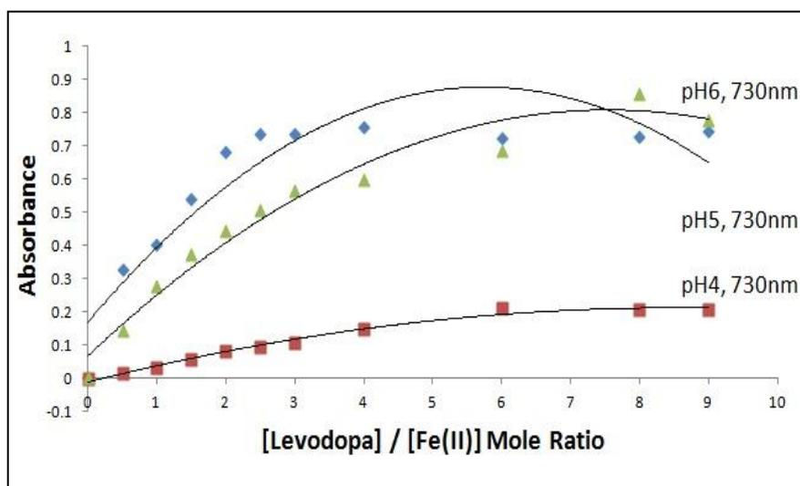
**Fig-9:** Stoichiometry of Fe (II)-Levodopa Complex, pH 4.0, 5.0 and 6.0. Fe (II) = 0.005 mmol.  $\lambda = 730\text{nm}$ .
