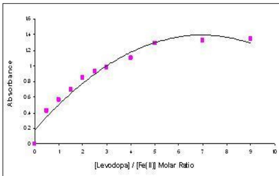
**Fig-6:** Stoichiometry of Fe (II)-Levodopa Complex in non-buffered aqueous solution. Fe (II) = 0.005mmol,  $\lambda = 730\text{nm}$ .
