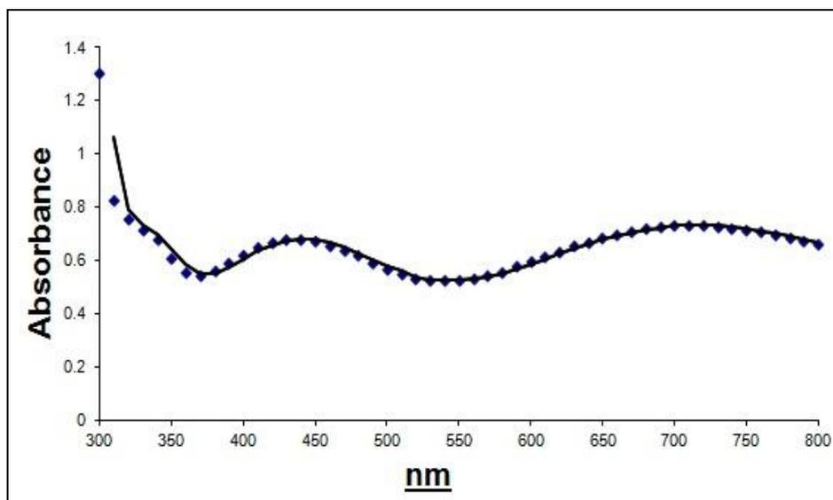
**Fig-2:** Spectra of Fe (II) complexed with Levodopa in non-buffered aqueous solution. Fe(II) = 0.05mmol, 10 fold ligand solution
